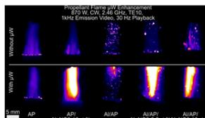
Left: Video of microwave-augmented combustion of composite solid propellants (several formulations), aluminized and unaluminized containing sodium nitrate dopant. 1 kHz light emission acquisition
