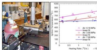
Left: windowed, vessel for combustion/ignition experiments. Right: High-speed ignition temperature measurement of a thermite in high-pressure air
