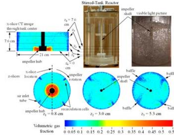
X-ray CT imaging of a 21 cm diameter gas-sparged stirred-tank reactor showing the local time-average gas holdup in a vertical slice through the STR center plane and several horizontal planes.
