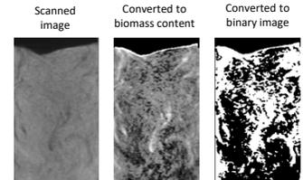
X-ray CT imaging to quantify mixing and segregation in binary (biomass-glass beads) granular systems.
