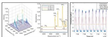
Above: Left, center: IR absorption speciation of evolved gas products from heating of a thermite. Right: Time-resolved quantum cascade IR absorption of methanol.
