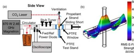
Above: Diagram of microwave augmented combustion cavity (left) and electric field distribution within the cavity (right).
