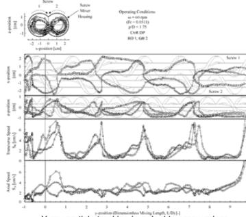
X-ray particle tracking in a double-screw mixer.
